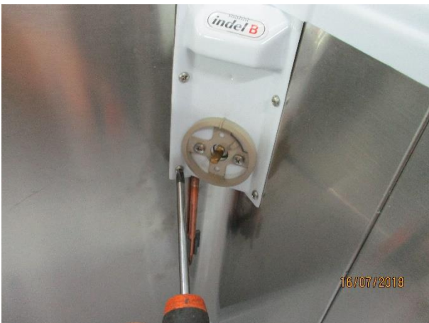
3. Unscrew the thermostat's box (4 bolts)
