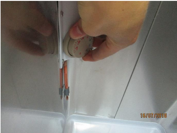
1. Remove the thermostat's knob
