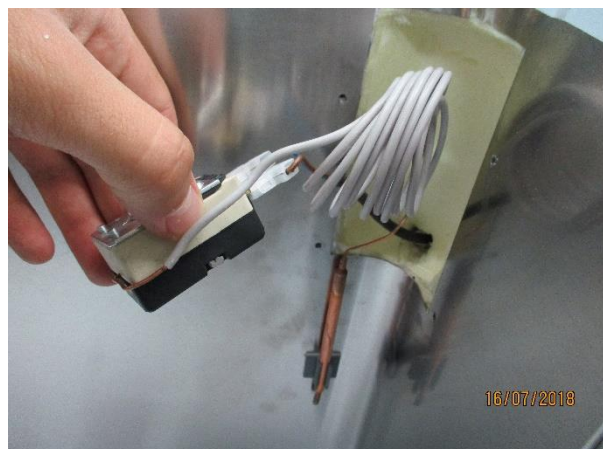
5. Pull the thermostat to remove it and reverse the procedure to replace the thermostat
