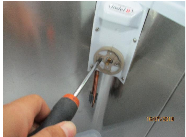
2. Unscrew the element fixing the knob (2 bolts)
