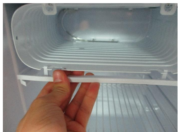
6. Remove the plastic protection
