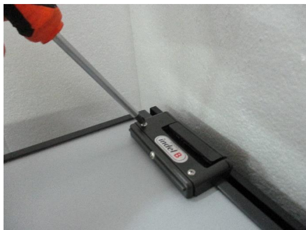
4. Remove the handle (3 screws)
