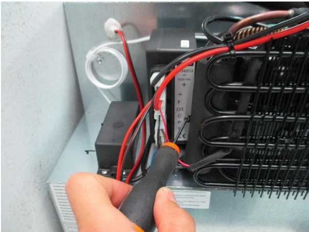
1. Unscrew the bolt fixing the ECU
