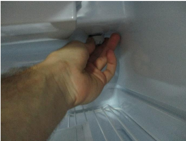
1. Remove the knob of the thermostat (pull it down)
