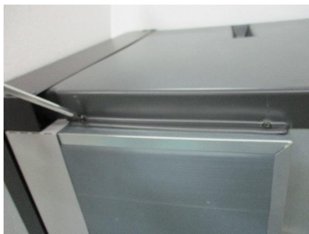
6. Unscrew the protection lid (5 screws)
