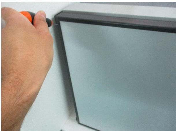
1. Use a thin object as a lever to remove the frame
