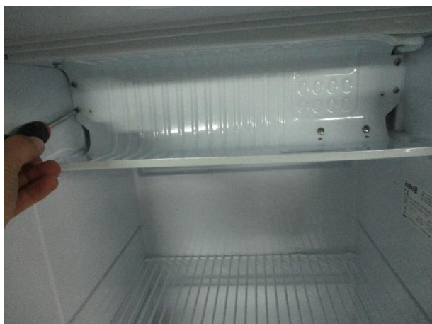
3. Unscrew the evaporator (4 bolts)
