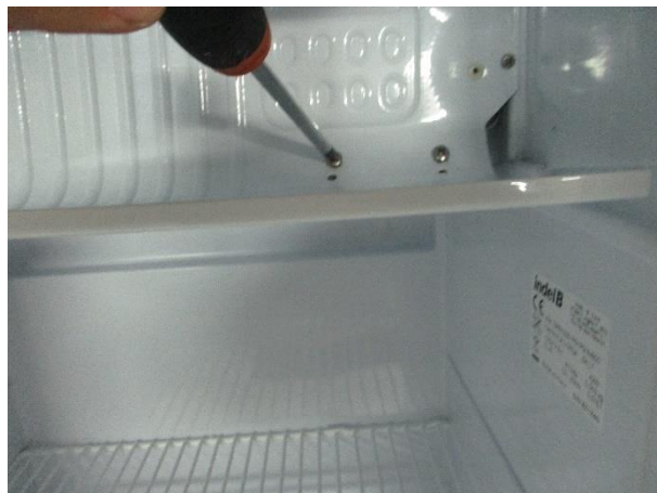
2. Unscrew the thermostat bracket (2 screws)
