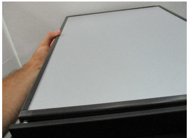
6. Lift the door from the opposite side of the screw nut to remove it, and remove the screw nut
