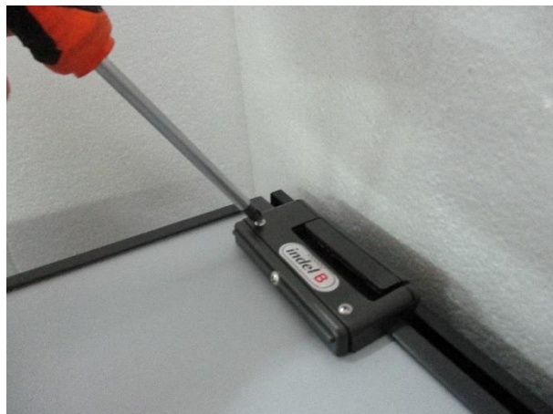
2. Unscrew the handle (3 screws)
