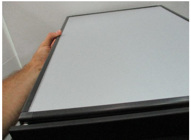
4. Lift the door from the opposite side of the screw nut to remove it, then reverse the procedure to replace it
