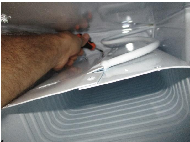
5. Unscrew the 2 bolts fixing the thermostat
