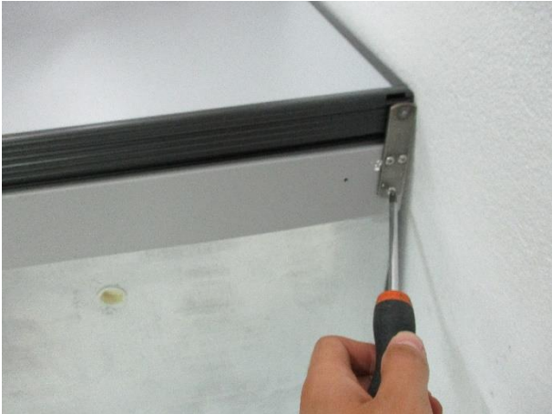
1. Unscrew the 2 hinges (6 bolts)
