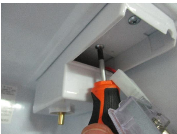
9. Unscrew the protection box (2 bolts)
