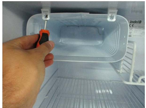
4. Unscrew the 2 bolts fixing the freezer
