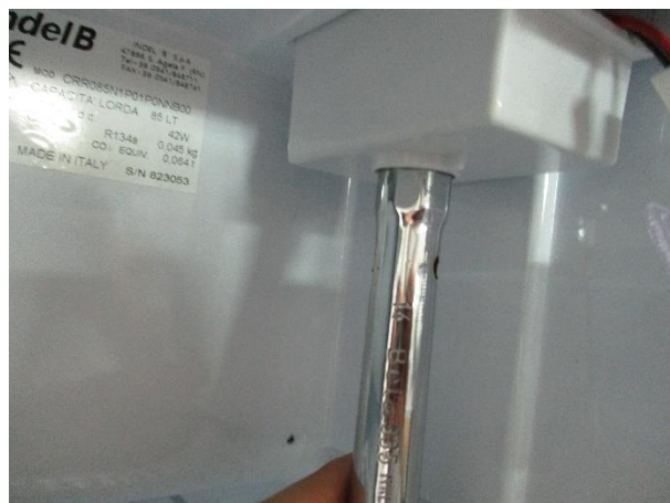
8. Unscrew the lock nut
