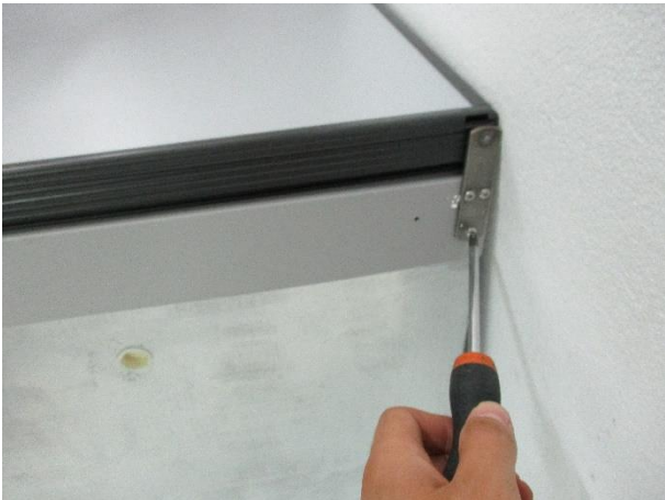
1. Unscrew the 2 hinges (6 bolts)
