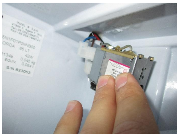
10. Disconnect the connection wires from the thermostat and pull the thermostat wire to remove it. Reverse the procedure to replace it
