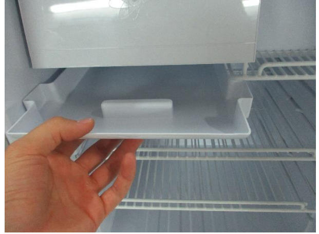
2. Remove the drip tray
