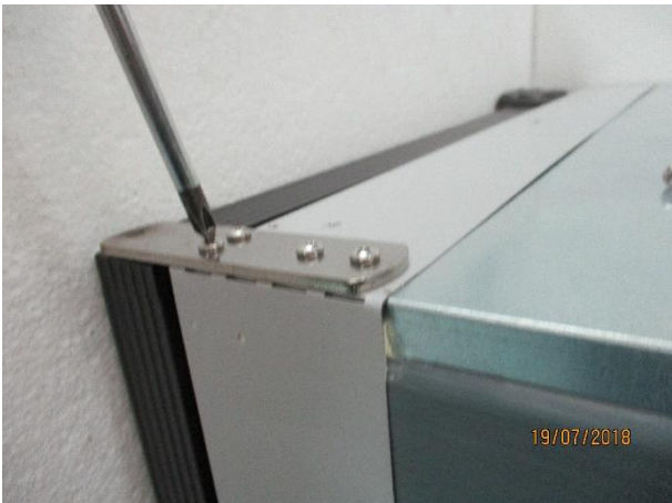
3. Unscrew the hinge (4 bolts)
