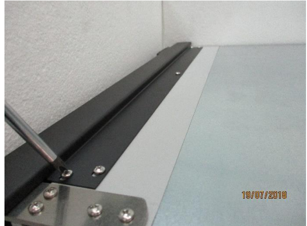
2. Unscrew the bracket (5 bolts)
