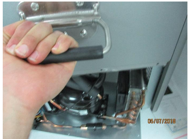
4. Lift the refrigerator and move forward the plate fixing the fan
