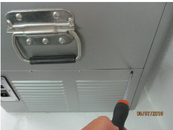
3. Unscrew the lateral bolts of the carter (4 bolts)
