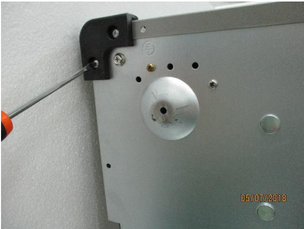
1. Unscrew the 2 corners (2 bolts)
