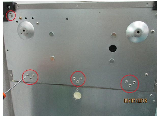
2. Unscrew the bolts fixing the bottom of the carter (12 bolts)
