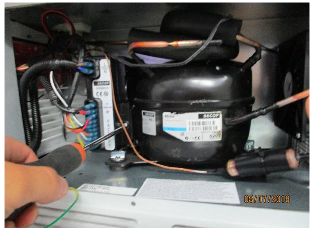
4. Unscrew the bolt that fix the ECU, disconnect all the wires and reverse the procedure to replace it
