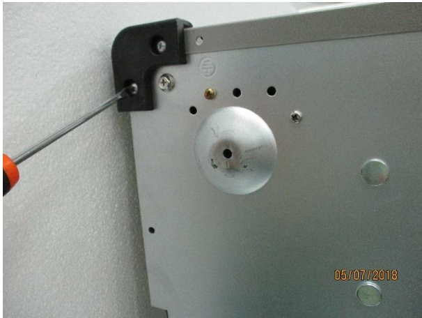
1. Unscrew the 2 corners (2 bolts)
