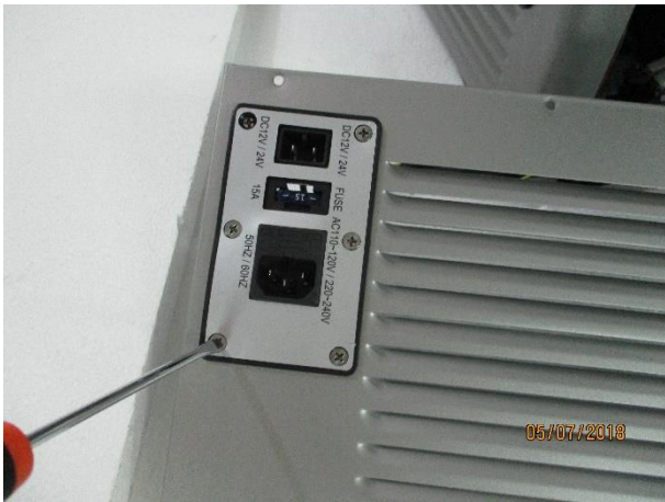
1. Unscrew the 2 corners (2 bolts)
