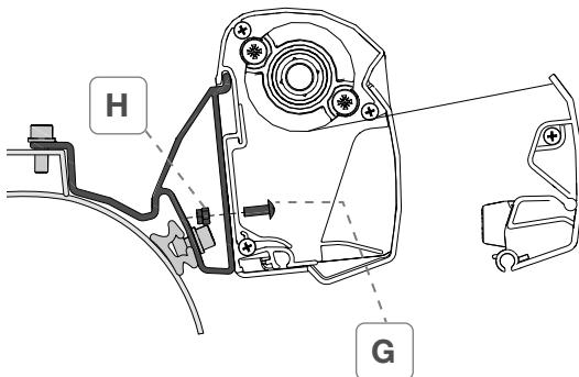
**EN** Before tightening the screws, make sure that the awning position doesn't prevent the opening of the rear door.
